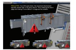
Automatically supress downstream equipment alarms with WebCTRL Fault Detection and Diagnostics (FDD), making it easier to diagnose problems.
