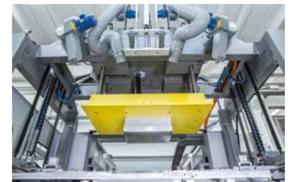
Upper mould plate (for pressure forming)
