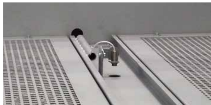
Optical pyrometer for monitoring heating and cooling
