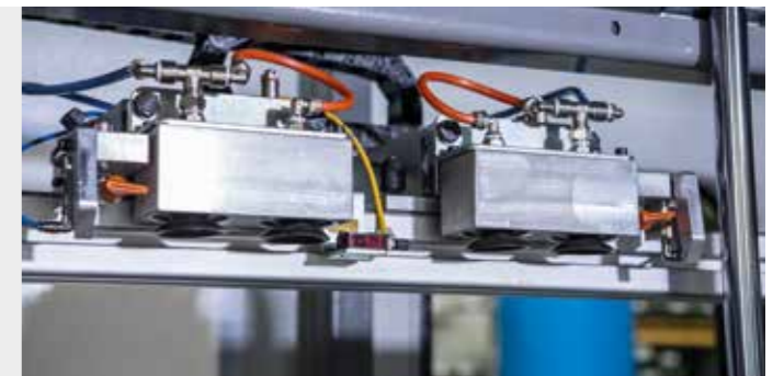
Automatic sheet centring system with double sheet detection
