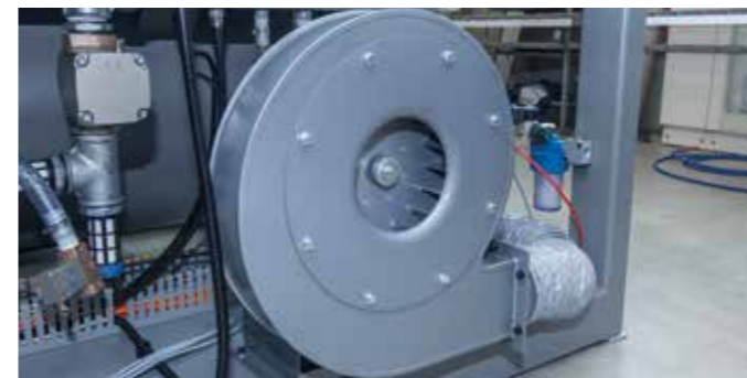
Electric fan for bubbling, vacuum and extraction
