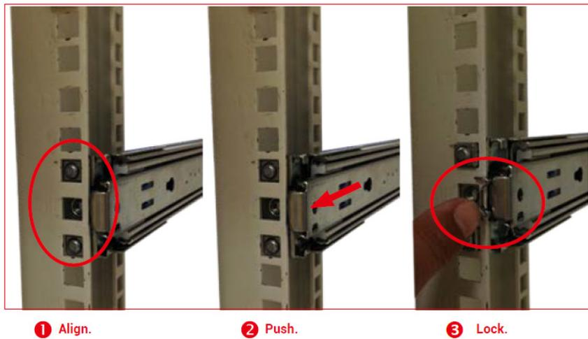
4. Verify that the ball bearing retainer is locked forward.
