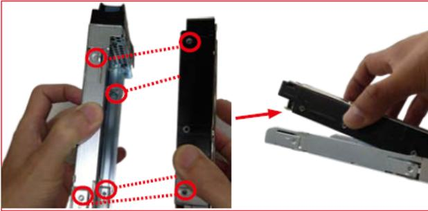
HDD can also be screwed on HDD tray by fastening two screws.
