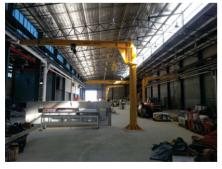
The JIB CRANE 360 is one of the most important elements in any mason's work shop.
