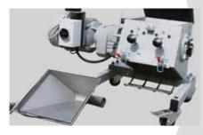
The quick snap system makes access to the cutting chamber, suction trough and screen area fast and easy. The hinged screen holder simplifies screen installation.
