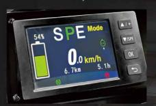
The multifunctional color-screen instruments are designed to have graphical interfaces and display data clearly. Three speed gears are provided to adapt to different operating environments. The interfaces can be switched and excellent ergonomic design. to be shown in Chinese and English to meet the needs of customers at home and abroad
