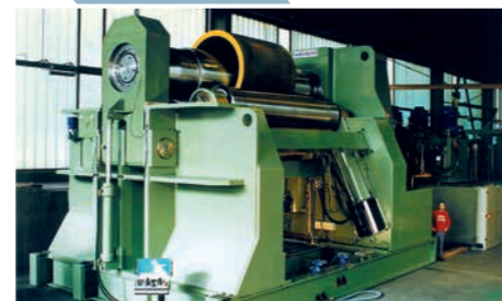
Plate width 4 000 mm, wall thickness 200 mm
