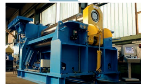
Plate width 3 000 mm, wall thickness 80 mm
