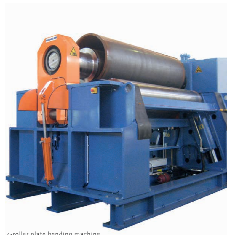
4-roller plate bending machine Type VRM-hy 3 000-610 Max. sheet width: 3 000 mm Max. wall thickness: 80 mm
