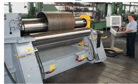
Plate width 2 100 mm, wall thickness 26 mm
