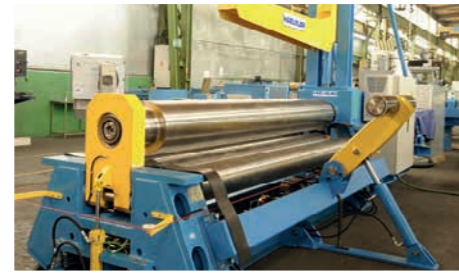
Plate width 3 000 mm, wall thickness 14 mm
