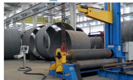
Plate width 3 000 mm, wall thickness 60 mm
