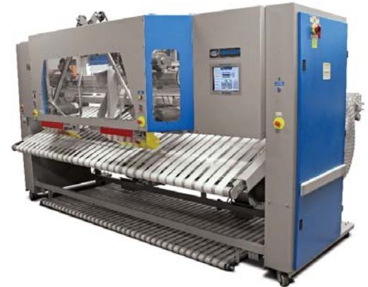
Bypass Conveyor In Raised Position For Use
