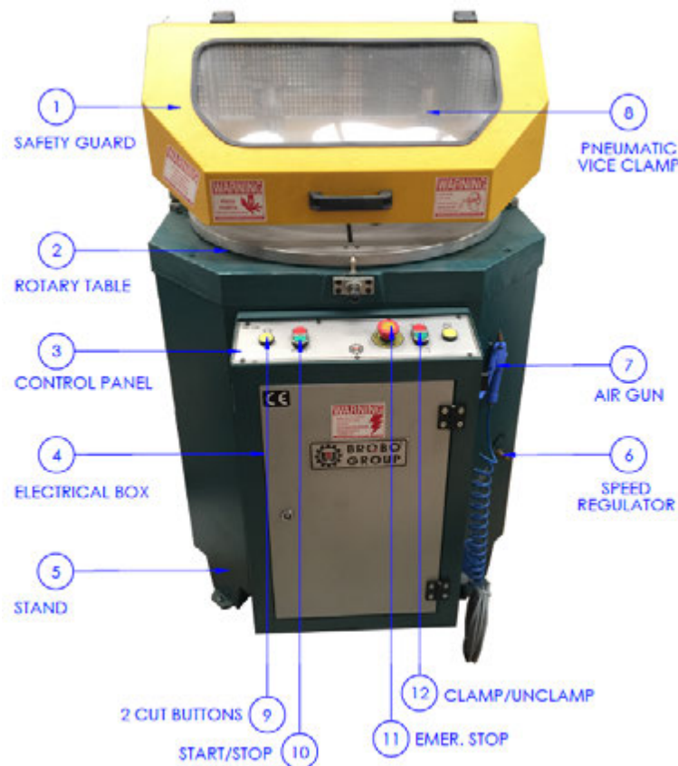
Figure 4. Up Cut Saw Main Components
