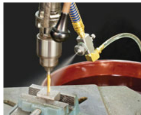
A Model 5R1010SS is used to supply a cooling mist for a drilling operation.
