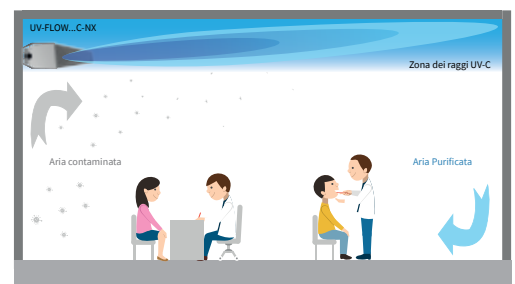
Disinfection of air upper layers
