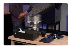
4. Dose powder: Use the scale to measure new and used powder and pour it into the Fuse Cartridge. Manually shake the cartridge for at least 1 minute, changing shaking direction multiple times, to ensure both are well mixed. The powder is now ready for your next print!
