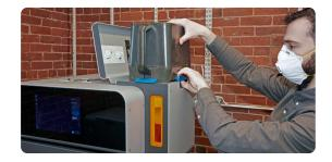
2. Insert a clean optical cassette: Removal, maintenance, and reinstallation of the optical cassette do not require any tools or disassembly. A second cassette enables you to run another print without cleaning one used for a previous print.
