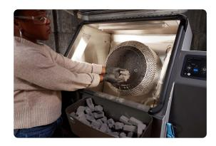
2. Set Up A Cleaning Cycle: The easiest way to clean your parts is to pick one of the preprogrammed routines. Choose the setting that best fits your parts, or adjust the settings of your cycles manually to match your part requirements. Click "Start" and let Fuse Blast do the work for you.
