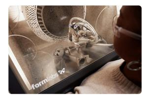
4. Change Media: In case of media saturation, or if you want to switch from cleaning to polishing, you will need to discard or change your media. For this, simply collect it by opening the valve over a container and running the machine for a minute.
