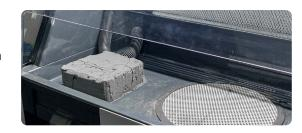
4. Extracting parts: Extract the parts from the cake of unsintered powder, breaking chunks by hand and shaking off the loose powder.
