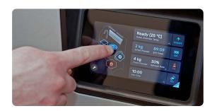
3. Ejecting the cake: Use the physical and virtual touch controls to raise and lower the print bed, allowing you to stagger the cake as it ejects from the build chamber into the Fuse Sift workspace. This is helpful for prints that contain a densely packed assortment of small or various parts.
