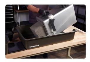
2. Extract parts & separate powder: Break the parts out fo the unsintered powder by hand. When using Fuse Blast for the cleaning step, you on only need to take 5mn to roughly depowder your parts. If you are using a manual media blaster or a model not equipped with media separation, you can scrub off the unsitered powder and semi-sintered shell with the included brushes and picks..
