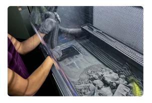
6. Reclaim Powder: Insert an empty cartridge into the drawer below the machine, then set the desired refresh rate on the interface and tap "Fill". Fuse Sift will automatically dose the new and used powder into the cartridge for your next print. Once the cartridge is full, remove it from the drawer and slide it onto the mixer on the right side of Fuse Sift then tap "Mix". Once this is complete, the powder is ready for your next print!
