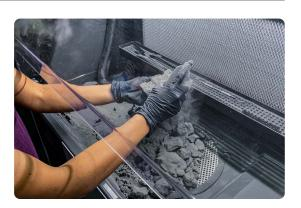
5. Cleanup: After extracting parts, begin cleanup. Powder that accumulates within the workspace can be wiped into the sifter and recaptured for later use. Smaller deposits around the workspace, within the build chamber enclosure, and on the hood can be picked up with the integrated vacuum hose for later disposal. The vacuum is controlled by a physical button conveniently located on the control panel.
