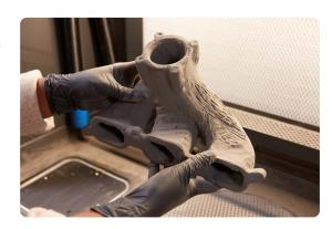
**5. Polishing:** Fuse Blast comes with the option to polish parts with a simple add-on. Simply insert the polishing system into Fuse Blast and switch your media to the Formlabs polishing media, then select a cycle or choose your custom settings.
