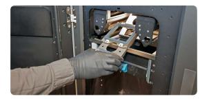
3. Insert a build chamber: Carry the build chamber between the printer and Fuse Sift using its integrated handles, no casters or support frames necessary. Having multiple build chambers in your workflow enables you to run another print while a previous one is still cooling.
