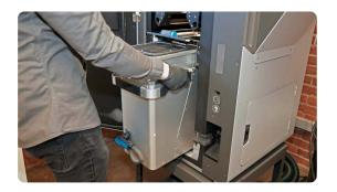
4. Connect Nitrogen Supply (Fuse 1+ 30W only): If your material requires an inert gas environment, connect your nitrogen supply to the back of your printer, then tap the printer icon in the left sidebar to access the printer status screen and toggle "Nitrogen System" to ON. Confirm that the touchscreen shows "N2 Mode" and that both the Inlet Pressure and the Valve Pressure are in range.
