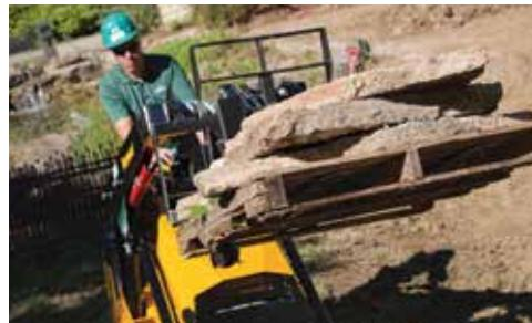
**ADAPT TO THE CHALLENGE.** The option of a wide 9" (22.9 cm) track or a narrow 7" (17.8 cm) track and a universal mounting plate allows you to work with a variety of attachments on the job.
