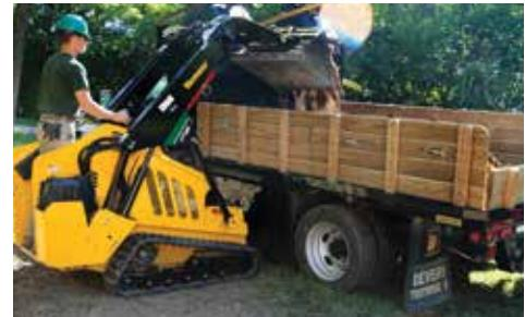
**HIGH STANDARDS.** The CTX100 comes standard with a dual hydraulic system capable of providing 15.5 gpm (58.7 L/min) of hydraulic flow to power the most demanding attachments, and low flow offers 8.1 gpm (30.7 L/min) to give maximum control.
