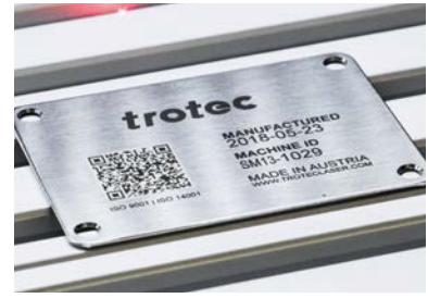
Annealing on stainless steel
