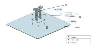
2. Fix the antenna on vertical steel frame or pillar with M8 \* 125mm screw, washer and screw nut.
