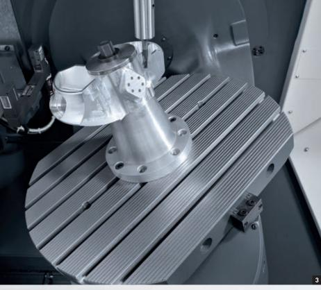
1: Flexible machining from three to five axes 2: Unobstructed view into the working area with optional tool magazine 3: Simultaneous table
