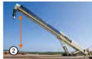
RazerTail Truck Unloader and TeleStacker® Conveyor loading Panamax vessel at 1,360 tonnes/hour
