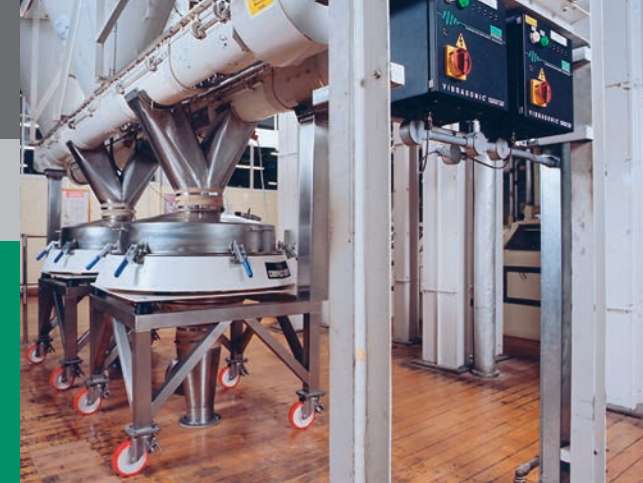
Compact 900 Sieves with Vibrasonic® deblinding system at Colmans - mustard powder producer. The screens are fed from blenders and pass the sieved material through to the packaging area.
