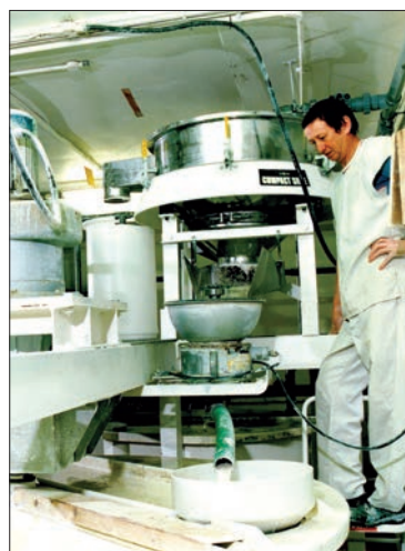
Compact Sieves are suitable for screening wet materials as shown here at Royal Crown Derby.
