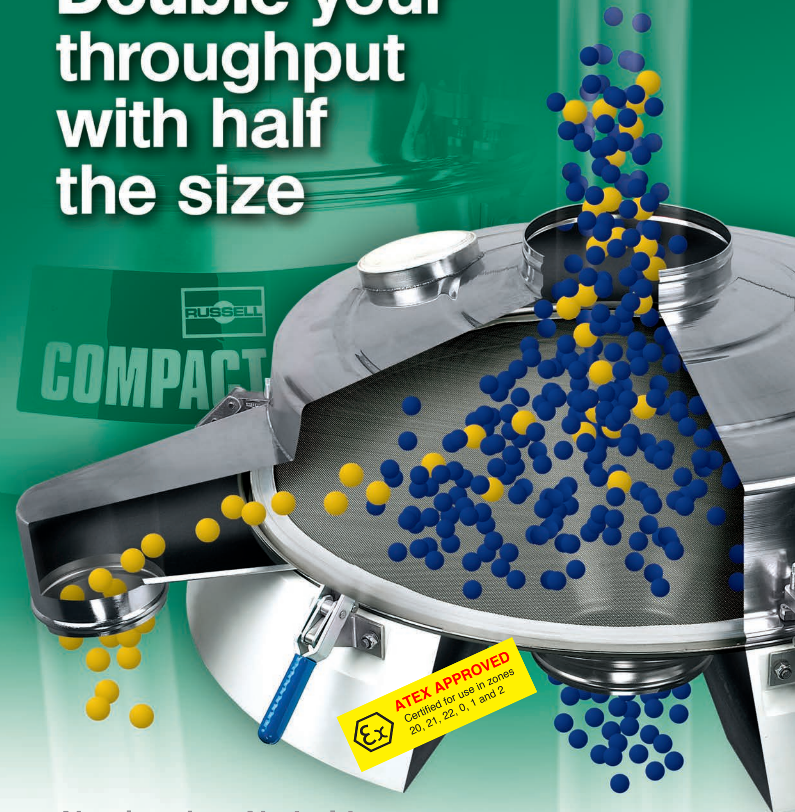
Compact 900 Sieves with Vibrasonic® deblinding system at Colmans - mustard powder producer. The screens are fed from blenders and pass the sieved material through to the packaging area.
