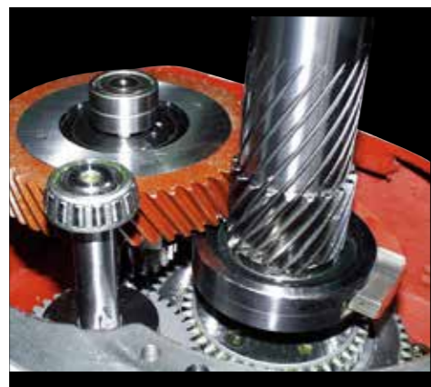
Strong back gear transmitting instead of timing belt for Hi-Low speed
