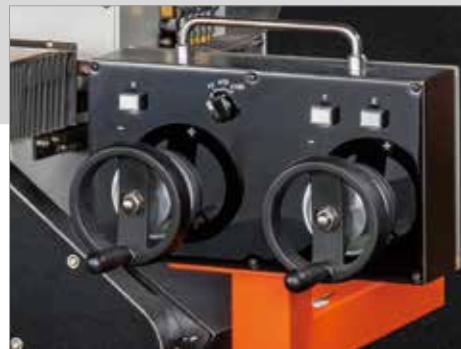
Electrical handwheel for X and Y axes provides easy operation
