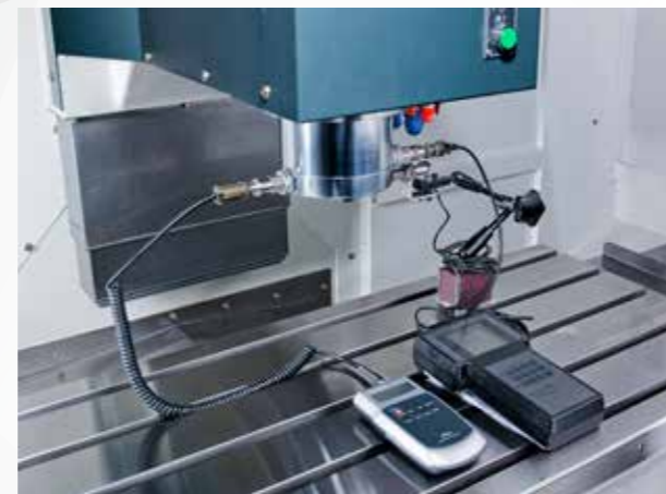
SPINDLE NOISE & VIBRATION CHECK
