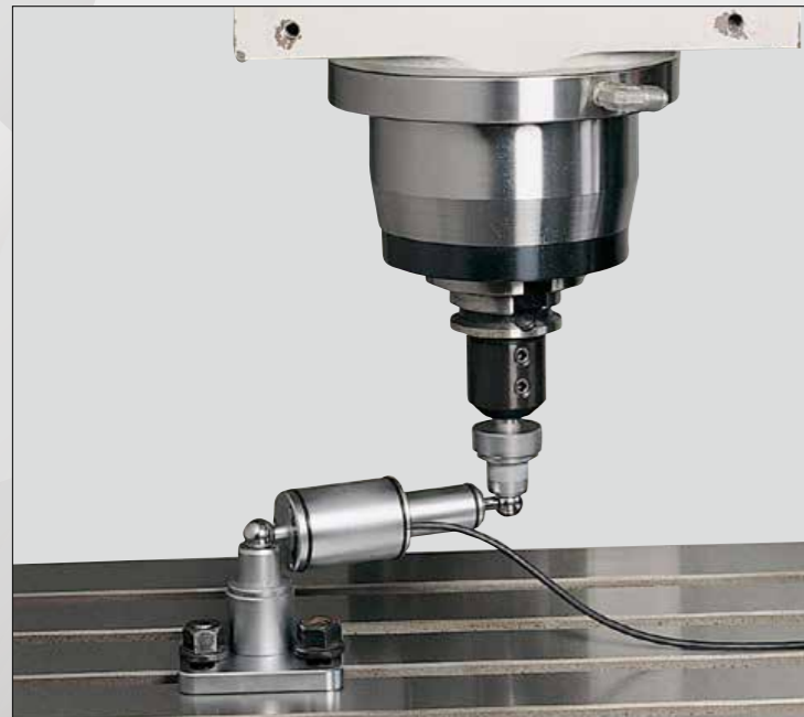
BALLBAR TEST Every machine is inspected by a ballbar test to ensure machining accuracy
