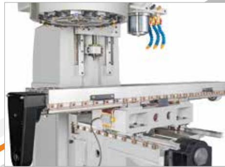
Linear guideways on XYZ axes
