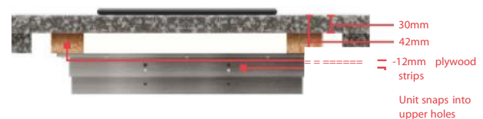
Figure 4: Incogneeto™ Unit Mounted to 30 mm Countertop with Two Plywood Strips
