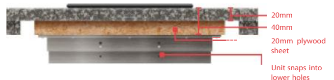
Figure 2: Incogneeto™ Unit Mounted to 20 mm Countertop with Plywood Sheet
