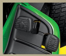
**Twin Touch System.** Twin Touch" automatic transmission lets you easily change from forward to reverse with two-pedal foot control for effortless speed and direction changes. (Available on Select Series Tractors.)
