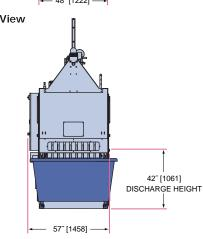
Versatile design allows use with a wide variety of carts or conveyors with a choice of input and output sides
