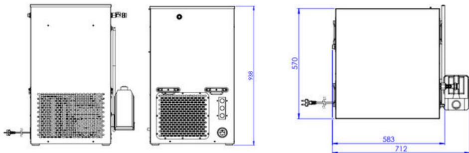
Our chillers feature a double-circuit insulated enclosure that accumulates high levels of refrigeration through the formation of ice in the tank water.
