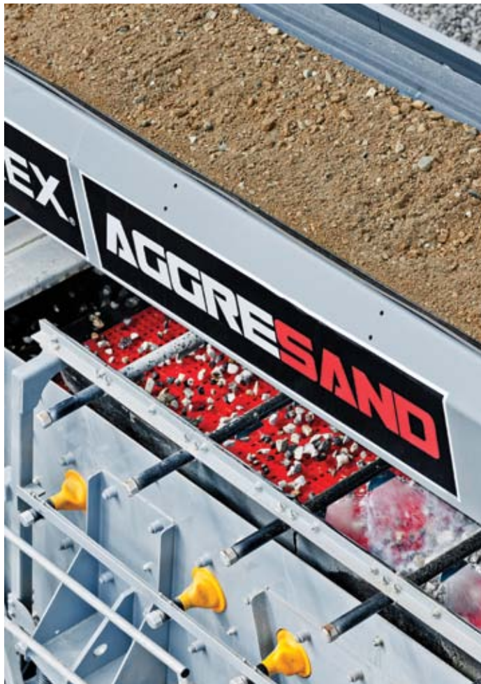
Aggregate Screen Fitted with Isolated Spraybars
