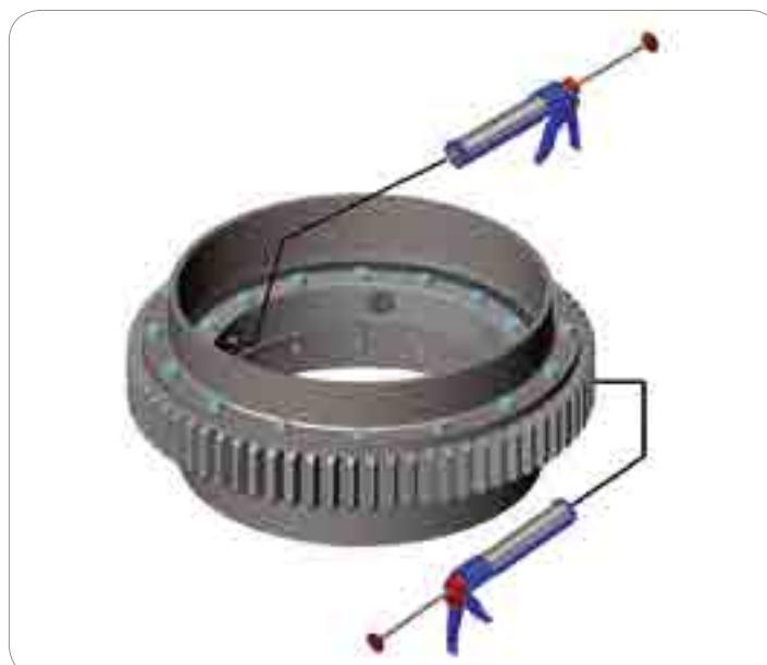
11. Lubricate the raceway using the grease fittings supplied in one of the bearing rings, and also lubricate the gear teeth (see Figure 9).
