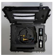
transportation. Sample lines and the most common DN8 and DN20 fittings are included. Alternative fittings are available to suit almost any  $SF_6$  installation.
