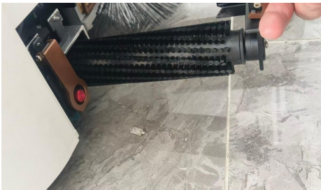
Scrubbing brush installation
