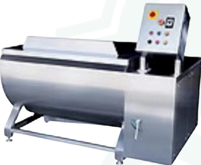
**Streamlined Batch Washing:** The TW02 uses a hydraulic tipper cradle for fast loading and controlled unloading, creating an efficient batch-wash workflow ideal for small-medium processing operations.
