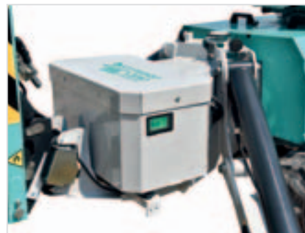
Lithium batteries compartment: protected and easily accessible for the charging cycle management. LCD display for charging status and remaining battery time.
