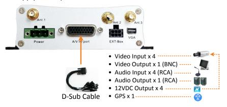
**Camera Connection:** Connect to the eZ.HD cameras using the four Video Input cables. To supply power to cameras, connect the 12VDC Output cables (500mA each) to the cameras. Note that the mobile DVR doesn't support HD-TVI / HD-CVI / HD-SDI cameras.
