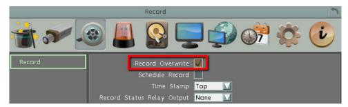
If Record Overwrite is not enabled, the recording to the SD card (general recordings or alarm event backup recordings) will stop when card space is full and the mobile DVR will automatically pop-up a message "SD Card Off" for notification. Users will have to replace a new SD card; or backup the SD card recordings and then erase (format) the SD card to resume the recording.
