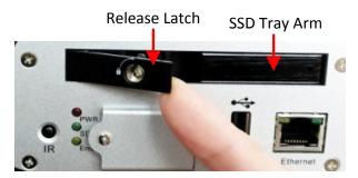
3. Insert an SSD into the SSD tray.
