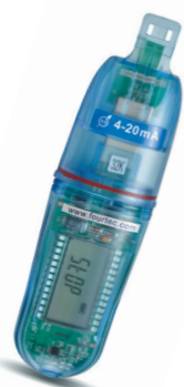
External 4 to 20 mA input LITE5032L-4/20
