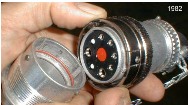
Fig.VM1 VRT breakaway connector.
