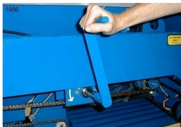
Fig. C5 Calibration handle rotates anti-clockwise.
