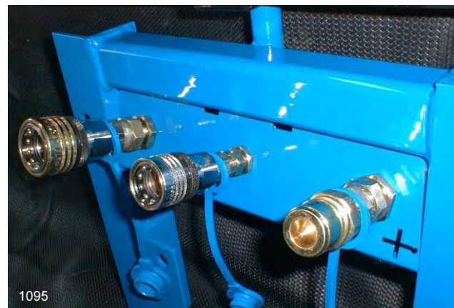
Fig. H6 Implement Hitch with Tema couplings.
