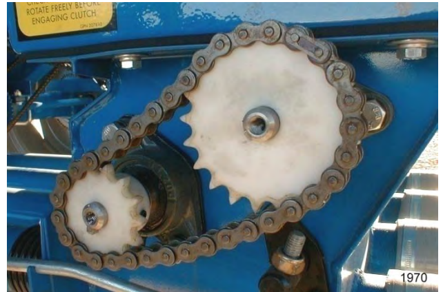
Fig.MD4 High Rates Sprocket Ratio.
