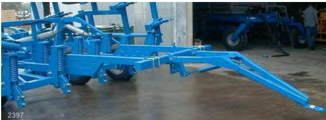
Fig. A7 CTC A-frame supported by spring mechanism
