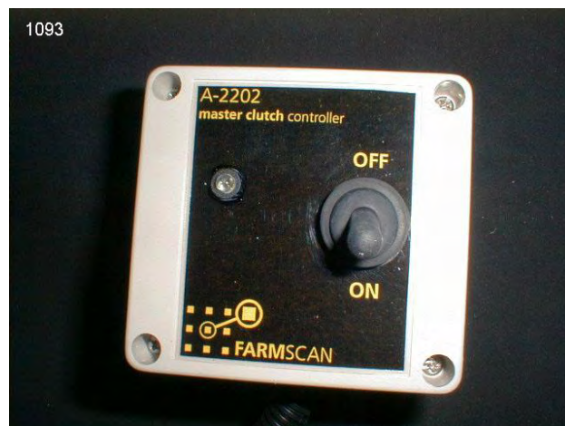
Fig. G2 Clutch Switch (single shown).
