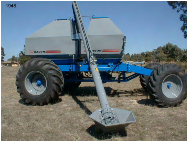
Fig. AO1 2120RT with auger in filling position.
