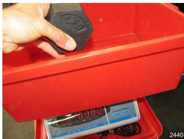
Fig. GM3- Scale Test Weight being used.
