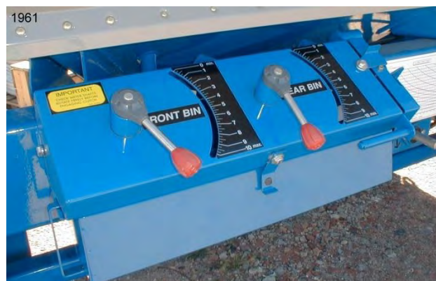
Fig. MD2 Variator Adjustment (2 bin).
