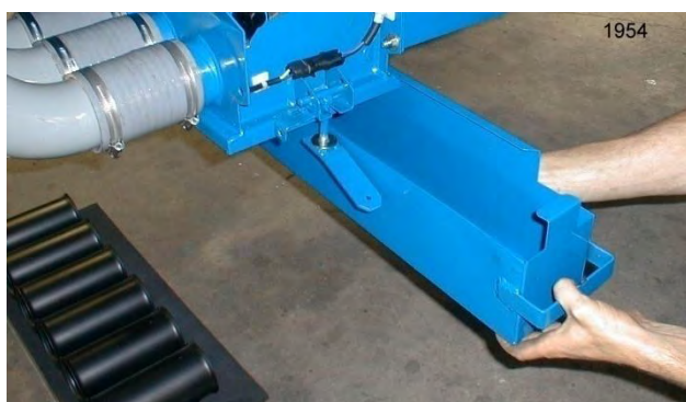
Fig. C3 Fitting the calibration collection box.
