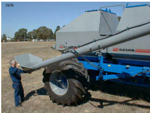
Fig. AO5 Manoeuvring the auger.
