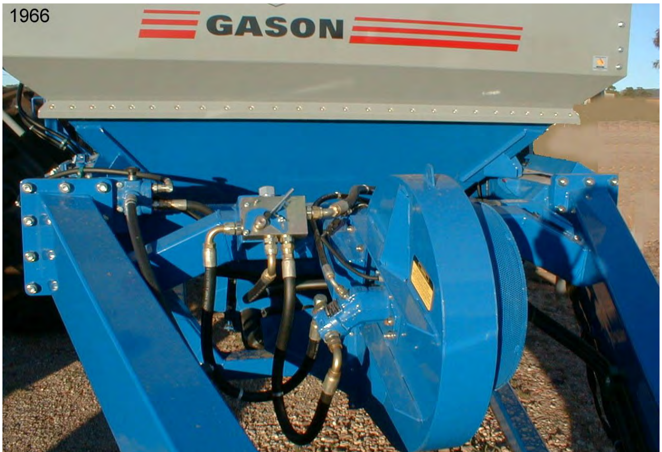
Fig. B4 Blower Assembly fitted to 1880FT Air Seeder.
