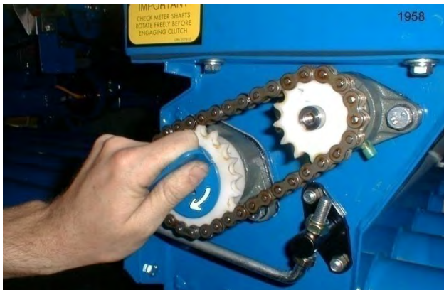
Fig. MD3 Checking Metershaft.
