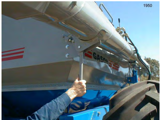
Fig. AO4 Rear auger barrel clamp.
