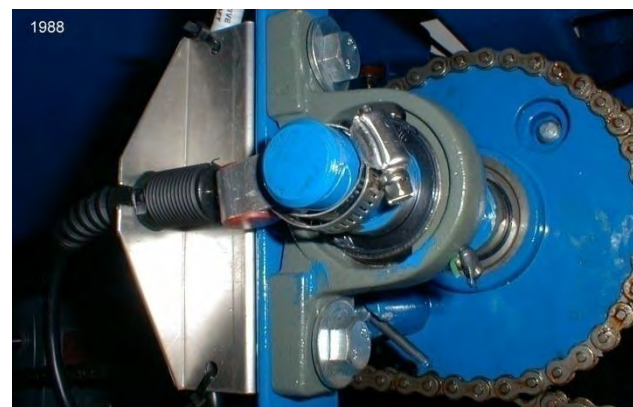
Fig. C9 Drive wheel magnet and sensor.
