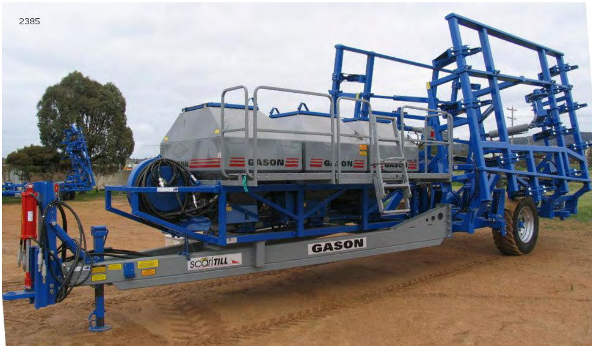
Fig. 2 1230 IM3 Series Air Seeder Mounted on CT2 Implement
