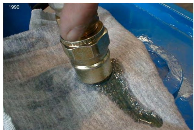
Fig. H7 Draining a small amount of oil.
