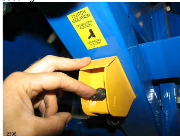
Fig. C10 Master Clutch Isolation Switch on a 3 bin G/Drive seeder.
