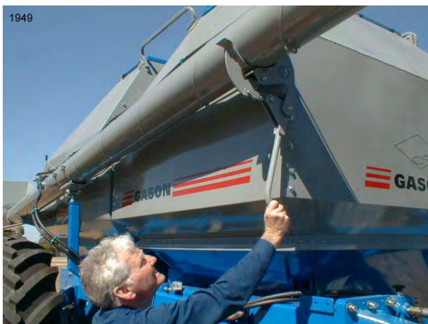
Fig. AO2 Front auger barrel clamp.
