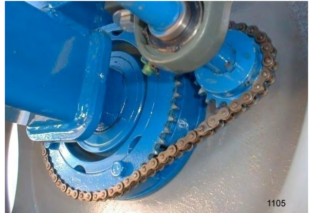
Fig.T1 Wheel Sprocket on a Ground Drive model.
