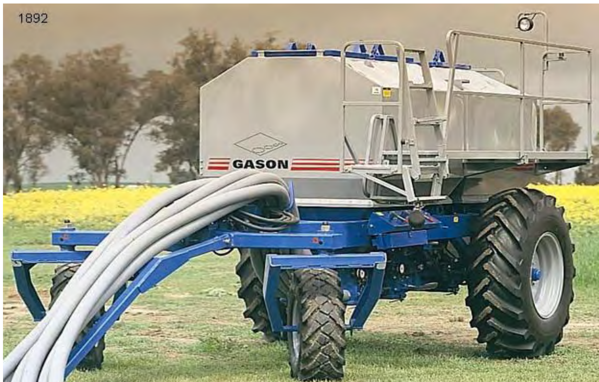
Fig. S2 1850RT Series Air Seeder CT (control traffic) Option.
