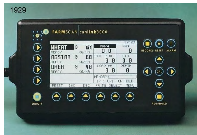
Fig.V1 The Canlink 3000 monitor .
