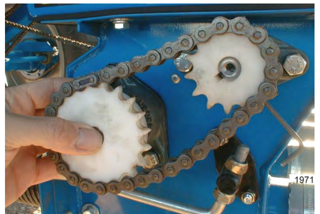
Fig.MD5 Standard Sprocket Ratio .
