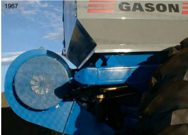
Fig. B1 – Blower Assembly
