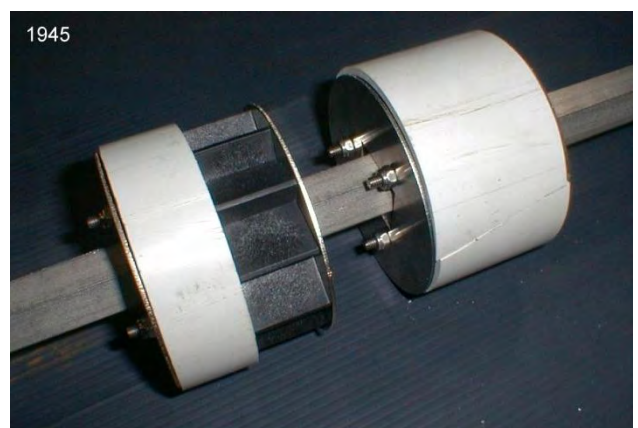
Fig.M15 25 & 50mm reducing sleeves on 6 outlet meterwheel assemblies.
