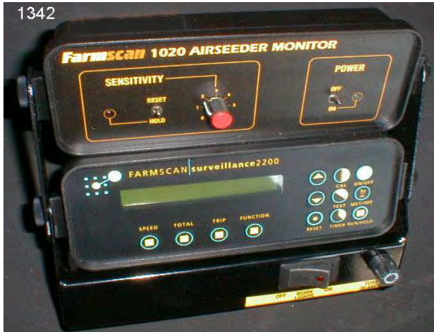
Fig.G1 Ground Drive Seeder Monitors and worklight switch bracket.
