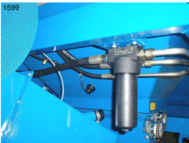
Fig. H8 Hydraulic Oil Filter.
