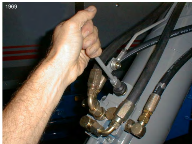
Fig. AO7 Directional Control Valve.
