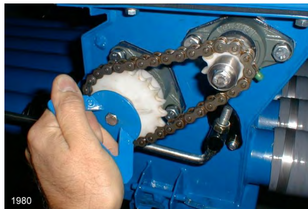
Fig. VC9 Removing the retaining collars.
