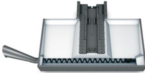
**Single Auger** All Haas VMCs are available with a single, auger-style chip conveyor that automatically removes chips from the machine, while compressing them and wringing out the coolant. For added reliability, the system reverses automatically if a jam occurs.
