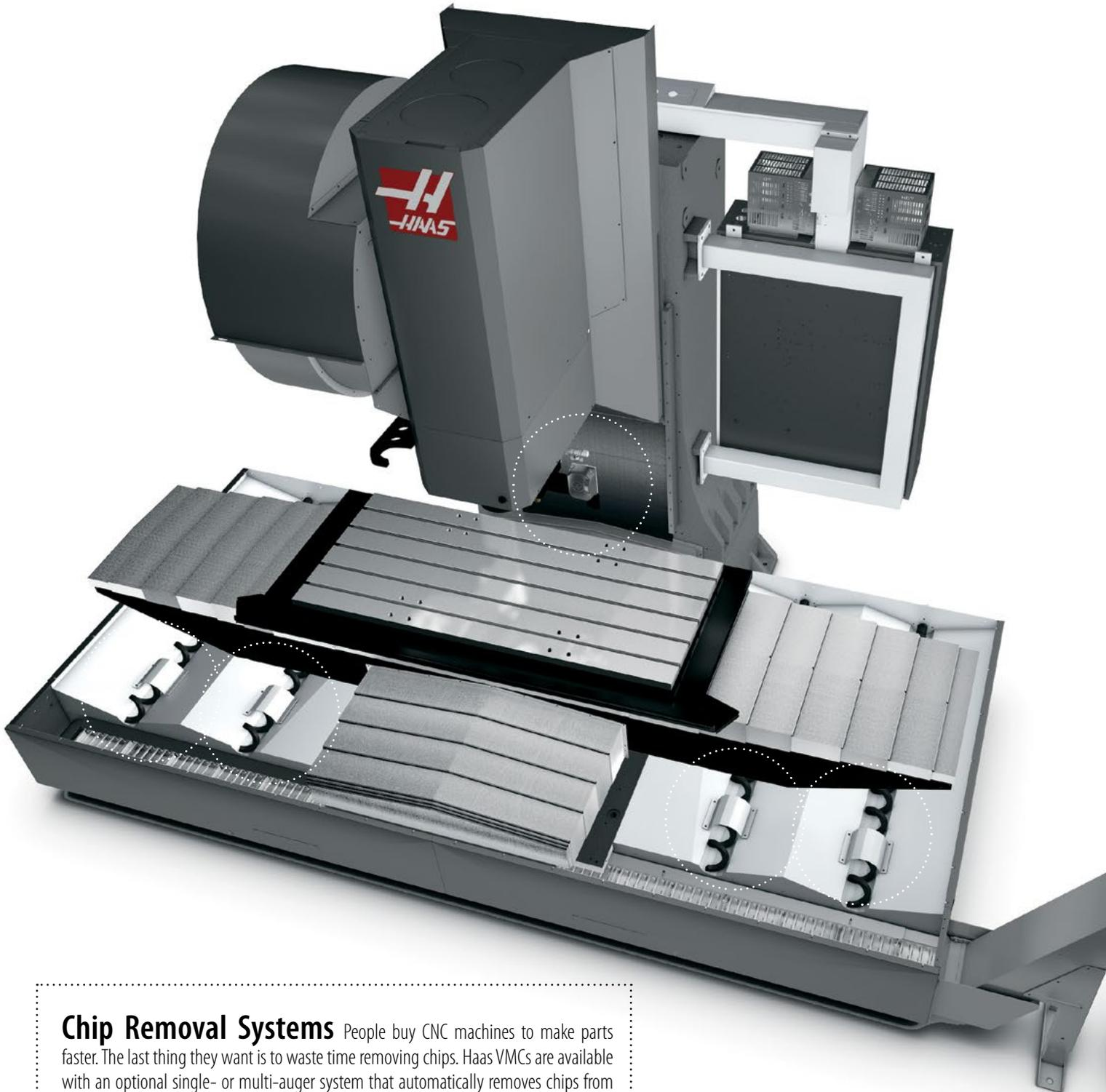
**Chip Removal Systems** People buy CNC machines to make parts faster. The last thing they want is to waste time removing chips. Haas VMCs are available with an optional single- or multi-auger system that automatically removes chips from the enclosure and conveniently discharges them at the side of the machine.
