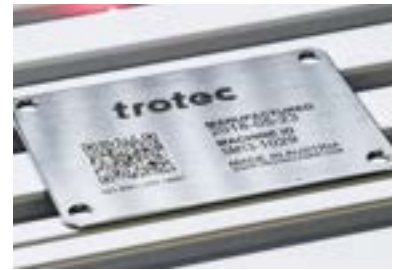
Annealing on stainless steel
