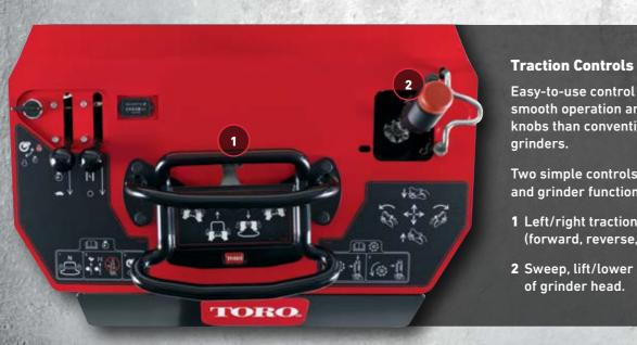
Easy-to-use control system offers smooth operation and fewer levers/ knobs than conventional stump
