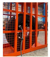
The explosive force released from a tyre fail during inflation results in a destructive air blast with particles propelled long distance at great speed
