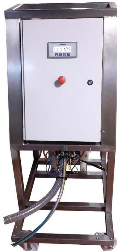
Innovet Controls supplies a portable system that can be wheeled (or pushed) next to the tank where the filling is to be done. The filling hose has a nozzle assembly fitted to the end of the hose. This nozzle assembly incorporates start and stop push buttons which start and stop the filling system.
