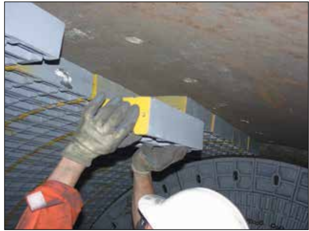
A magnet holds the liner to the drum.
