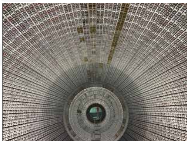
A typical MML installation for a 16.5'X37.5' mill
