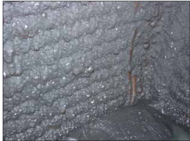
The ball chips are attracted to the liner and form a protective layer.
