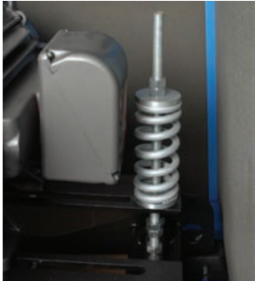
Automatic V-belt drive tensioning system.
