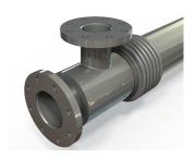
The HRS DTI Series is a complete stainless steel double tube heat exchanger designed for industrial and environmental applications. The product flows through the inner tubes and the service fluid flows through the surrounding shell. As a result of its geometry, the DTI Series has a continuous free-pass cross section allowing large particles to be processed and reduces the risk of product blockages.
