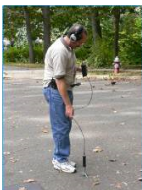
Fig.5 using the tripod attached to the hand probe microphone
