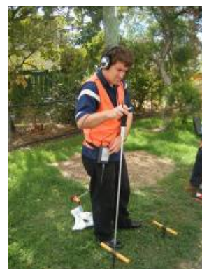
Fig.4 listening to the pipe via an insulated toughened probe
