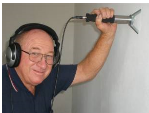
Fig.6 listening to a leaking pipe through the wall
