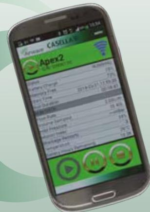
Start, stop and monitor the pump remotely via an iOS or Android device.
