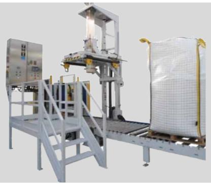
The Ilerbulk is a big bag filling station for 1 or 4 hook bags that can be adapted to the specific requirements of each industry. It has different grades of automation depending on required outputs and a dosing system on top depending on the product to be bagged.
