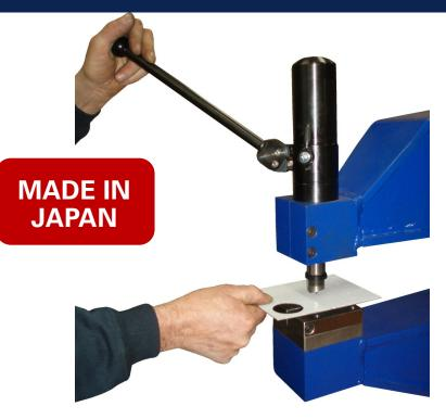
The EG3-600 hydraulic punch is ideal for sheet metal fabricators, repair workshops and electrical manufacturers. The EG3-600 punches round and square holes in sheet metal, stainless steel, copper, brass and aluminium. Dies and cutters can be easily changed in a matter of seconds. The unit has a locating centre-pin so the operator can punch holes accurately on the work piece.
