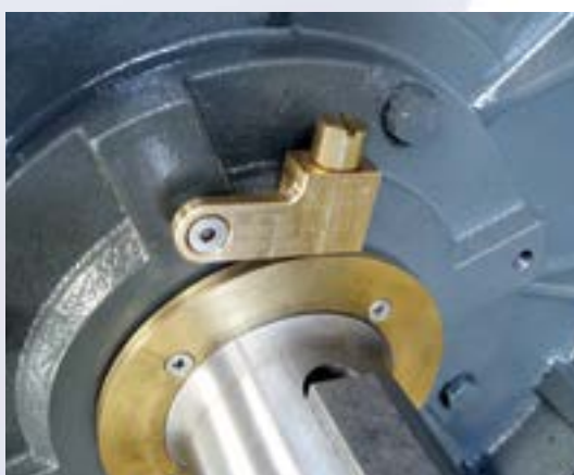
"Rotor Grounding Brush" fitted to D315 frame motor
