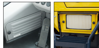
Inside air filter
