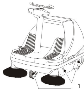
1 fastening bolts of side trim panel
