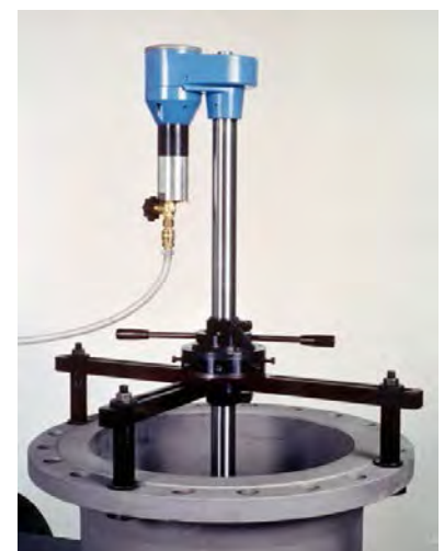
VALVA-2 with 3-point centre clamping
