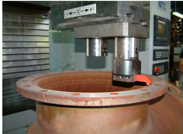
Face turning of flanges
