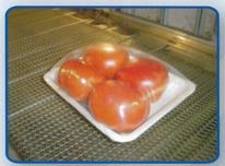
As product enters shrink tunnel the film initially expands stretching out all wrinkles
