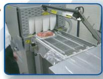
Seal bar releases and "bagged" product advances to shrink tunnel
