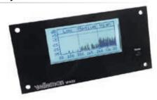
Features • 128x64px display • Measures RMS, peak power, mean dB, peak dB • Analyses linear audio spectrum and 1/3 octave audio spectrum • Auto or manual range • Peak-hold • Impedance selection • White backlit LCD • 12V DC powered • 300mW - 1200W @ 2 Ohm min range  $\, \bullet \,$  Suits 2, 4 or 8 Ohms, plus bridged amplifier option  $\, \bullet \,$  Easy panel mounting 98 x 51mm. • Just 35mm mounting depth!
